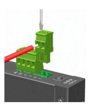
If cascading the power to next device is needed, install the power wires and plug for another switch. Then, use DC2 contacts.
