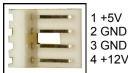
For aux power X5V and X12V (JP2), J2 must be connected to pc power supply! If not, the card wont work.
