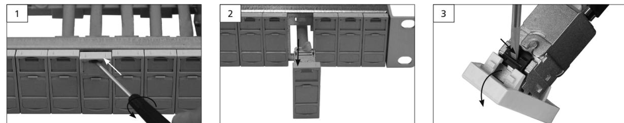
**D** Modulmontage Keystone 19 Zoll Modulträger 1HE Edelstahl / Mounting of Keystone modules to 19-inch module frame 1RU stainless steel /
