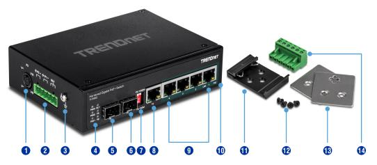
0 AC power port Terminal slot for DC power 2 3 Grounding point 4 LED indicators 6 **Gigabit SFP slot** 6 Shared Gigabit SFP slot 0 **Dip switches** 8 Shared Gigabit port 9 Gigabit PoE+ ports 1 IP30 rated metal housing 1 Din-rail mount Ð Screws B Wall mount kit Ť Terminal block
